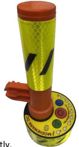
The **SELF TEST** button can be pressed at any time TO TEST the device is functioning correctly. All **LEDS** will light and a green light will indicate the device is ready. If a red light indicates change the batteries.
