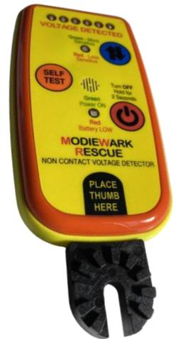
A **GREEN LED** will heartbeat to indicate the device is ready. If a **RED LED** light is indicated the batteries require changing.
