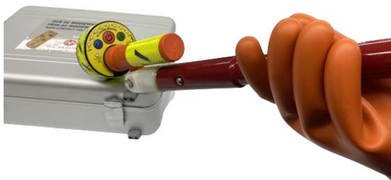
Before pointing the tester at the potential power source ensure you are standing with both feet grounded and the tester is not indicating any presence of electricity.
